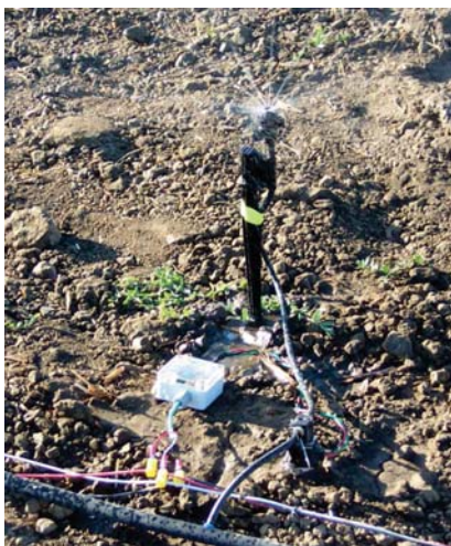
Individual microsprinkler with sensor would allow for site specific fertigation.
